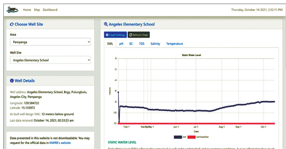
Screenshot of the PhiGO dashboard showing near real-time static water level in Pampanga based on a well located in Angeles Elementary School in Barangay Pulungbulu, Angeles City. Based on the dashboard, there are three other well sites in Pampanga.
