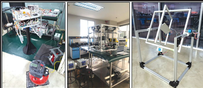
The visualization software for S4 or the Small Satellite Simulation System (top), which includes the hemispherical air bearing (lower-left), Helmholtz cage (lower-center), and motorized gimbal (lower-right).
