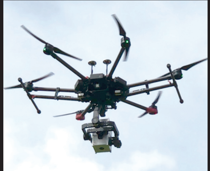
A flight test of the engineering model of Hypie, a push broom hyperspectral camera designed for drone platforms.
