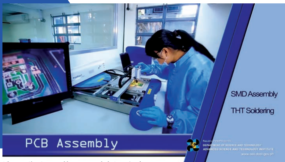
The EPDC's PCB assembly services include SMD (surface mount device) assembly and THT (through-hole technology) soldering.
