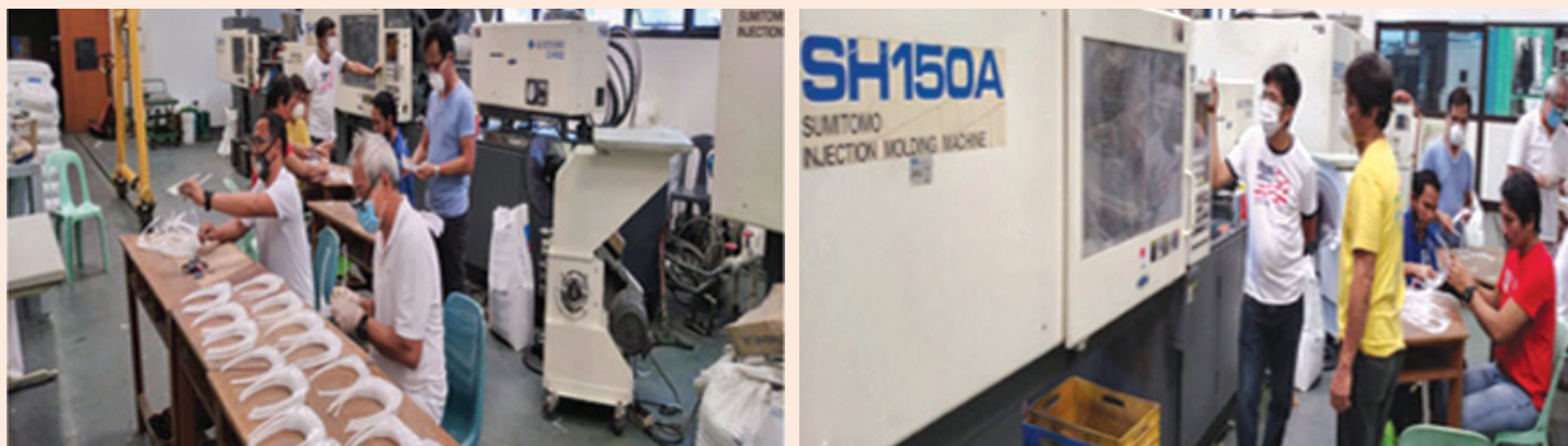
The plastic injection machine is housed inside the DMSC in the DOST-MIRDC Compound in Bicutan, Taguig (left); Team MIRDC engineers and technicians carry out mass production of the face shield frames (right). (Photos from DOST-MIRDC)
