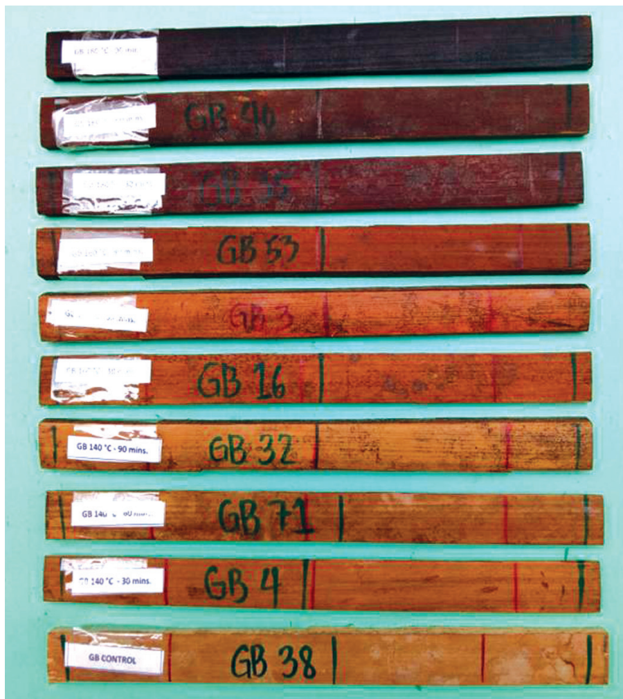
Researchers have studied the effect of TM on the strength of giant bamboo using spent engine oil as medium. Initial findings showed that TM made the bamboo more stable – less prone to swelling and shrinking. However, higher heat also made the material darker.
