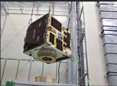
Solar Array Panel Deployment Test of Diwata-2 Flight Model. (Photo from PHL-Microsat)
