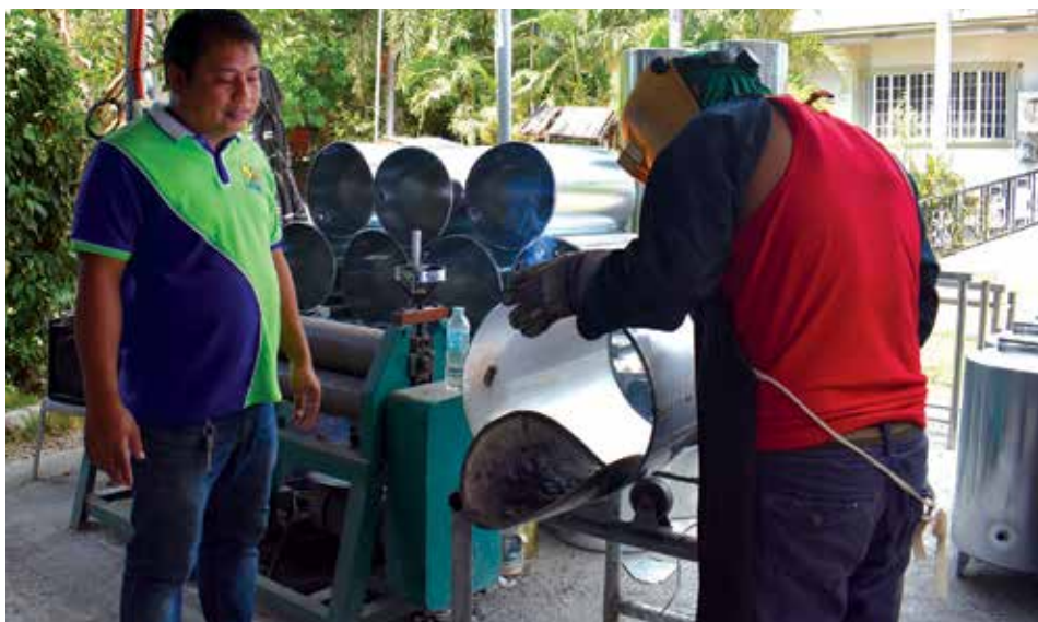
Mike V. Ruiz (left) supervises his staff to form a perfectly rolled water tank tube through the mandrel tube bender (beside Mike), a roll forming machine which he acquired through SETUP.
