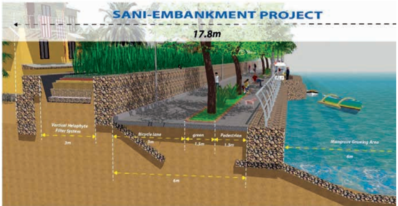
The helophyte filter system uses common reeds ( Phragmites australis ) and root bacteria as agents for treating the wastewater. (Photo from DOST-XI)
