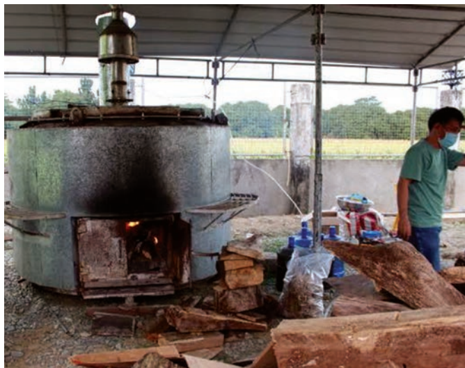
The improved bamboo charcoaling kiln can produce more bamboo charcoal and pyroligneous liquor than the old model.
