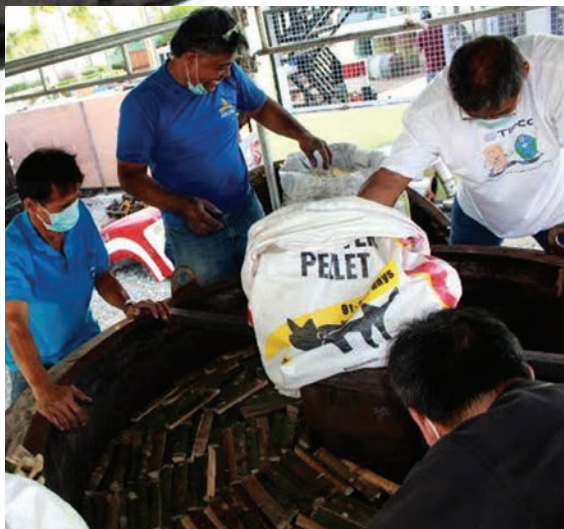
The improved bamboo charcoaling kiln can produce more bamboo charcoal and pyroligneous liquor than the old model.
