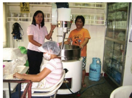
Clockwise: Top-left photo shows Corazon, the mother of Pamela G. Santos, manually cooking the tamarind candies under low fire using carajay and ladle. Top right photo shows the double jacketed kettle that BEAKRIS House of Goodies acquired through DOST's Small Enterprise Technology Upgrading Program which helped the firm to increase plant capacity and productivity, and improve the product quality. Right photo shows Pamela using the refractometer to measure the concentration of sugar, thus standardizing the sweetness of their products.
