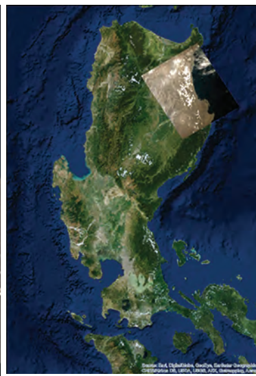
Left: A test image of the province of Isabela in the island of Luzon, the Republic of Philippines, taken by the medium field-of-view color camera (MFC), captured at 09:15AM Philippine time on May 17, 2016. The test image captures a portion of the coastal seaboard of Isabela province, which includes parts of the municipalities of Maconacon, Divilacan, and Palanan. Right: A projection of the image on the left. While taking this picture, the satellite was moving over Luzon island and was looking down vertically at the target area, with the pointing control toward the center of the Earth.
