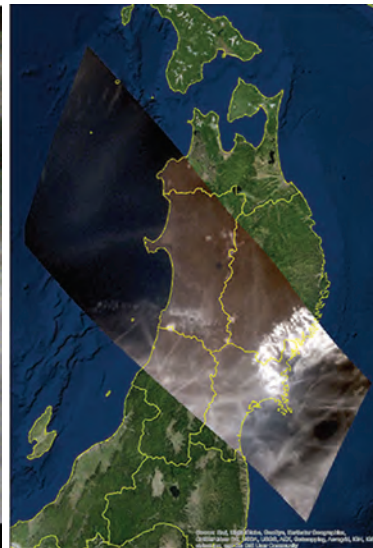
Left: An image of the Tohoku area of Japan taken by the medium field-of-view color camera on board Diwata-1, captured at 10:54 Japan Standard Time on May 9, 2016. Right: A projection of the MFC image of Picture 2 on a geological map of Japan's Tohoku region.
