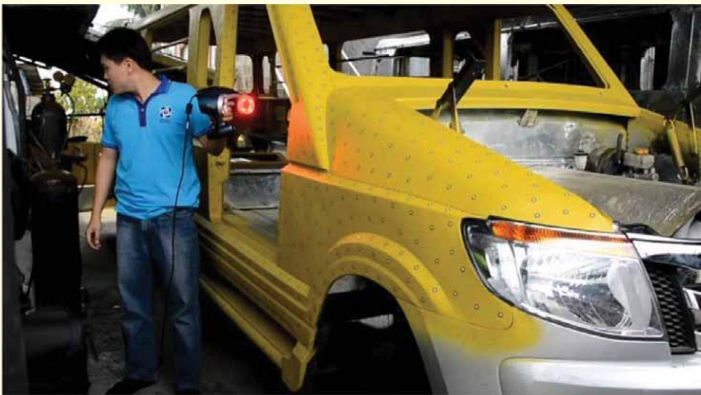
An engineer from Department of Science and Technology- Metal Industry Research Development Center (DOST-MIRDC) gathers necessary information of an Asian utility vehicles before it goes through Finite Element Analysis. FEA is a computerized method for predicting how a product reacts to real-world forces, such as vibration, heat, fluid flow, and other physical effects. (S&T Media Service/Photo by DOST-MIRDC)
