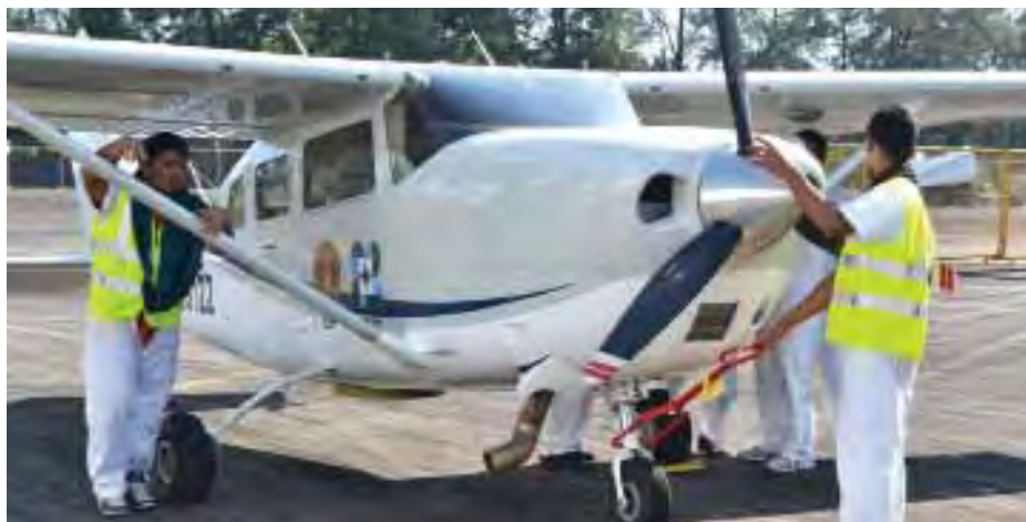
One of the DREAM LiDAR planes being used to survey the 18 major river basins in the Philippines (Photo courtesy of www.science.ph )
