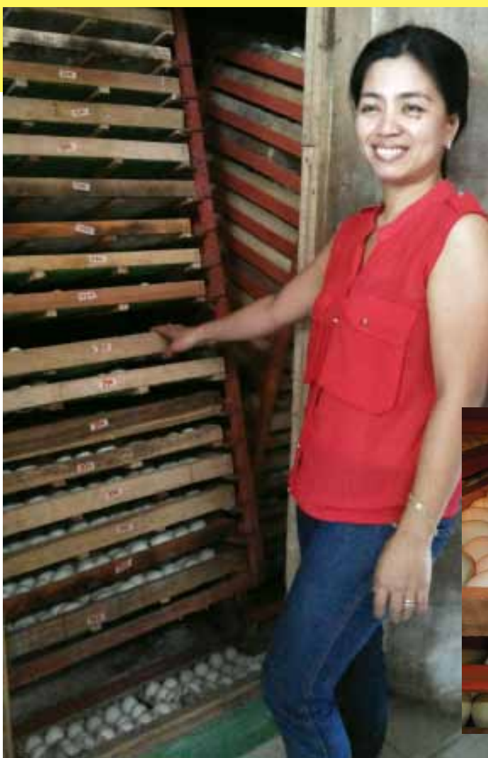
Maricris Huit and the automated 18-rack bay egg incubator with a digital thermostat control system.
