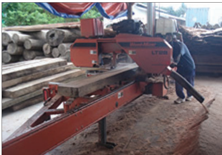
Confiscated logs by the DENR are being processed into lumber by DOST-FPRDI's crew using the Institute's mobile sawmill (below) before turning them over to TESDA, which constructs the lumber into armchairs for public schools (left).
