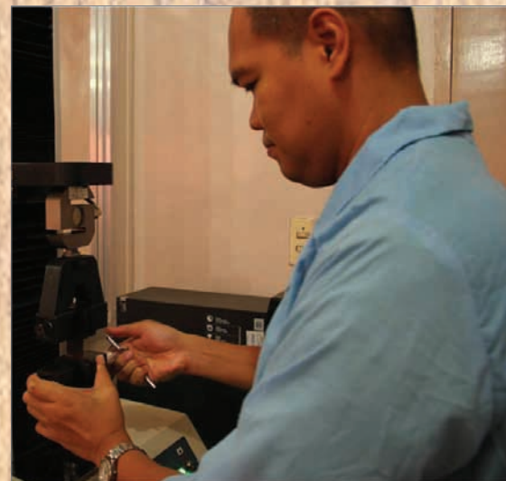
State-of-the-art equipment is used to test the plywood's shear strength.
