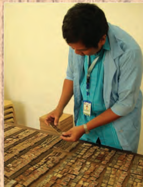
After subjecting the Type 1 plywood specimens to cycles of boiling, drying, and wet shear testing, a visual reading of wood failure is done to evaluate the glue bond quality.
