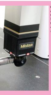
One of the knee implant components undergoes testing with the Coordinate Measuring Machine inside the OII facility. *(Photo by Henry A. de Leon, S&T Media Service, DOST-STII)*
