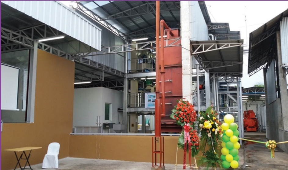
Prototype carbonizer (painted red) is shown in foreground. Behind it is the gasification component (fluidized bed gasifier). (Photo by RBSMC11)
