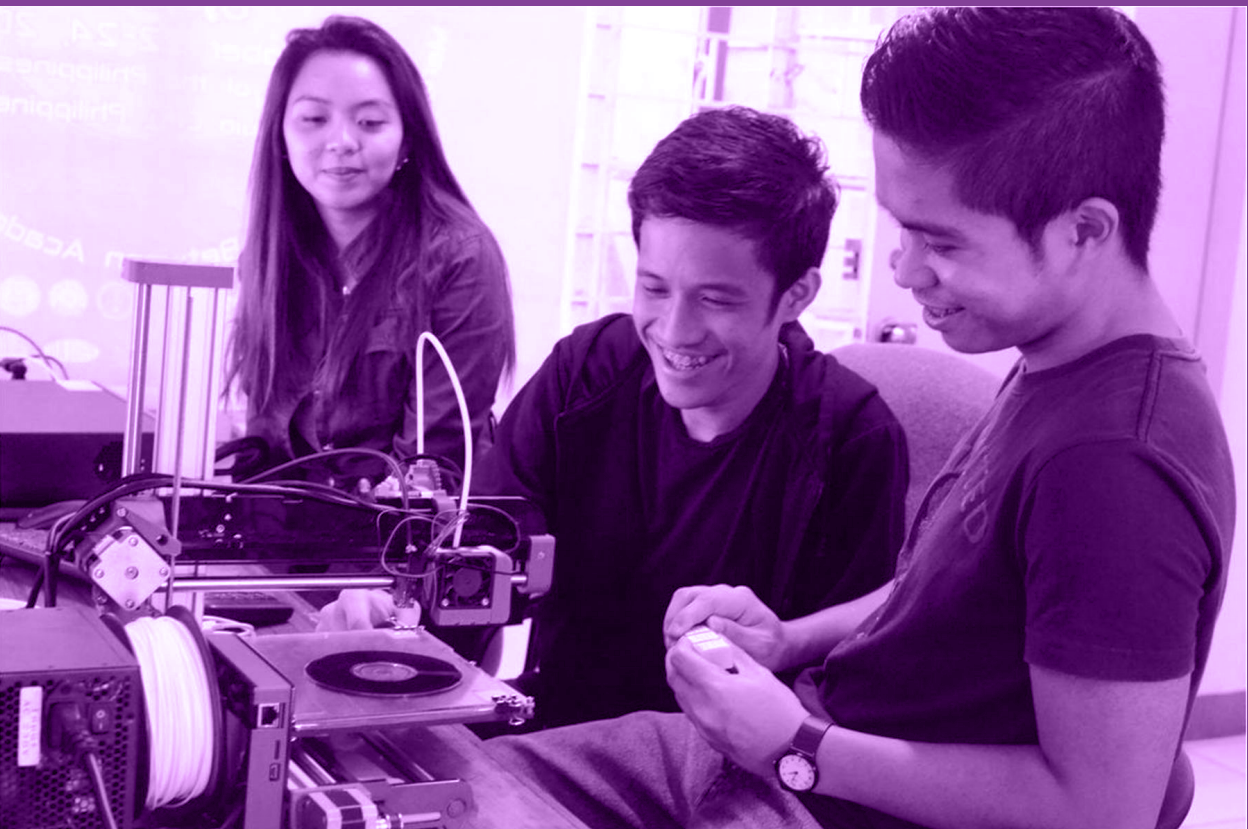
Graphene research team members (from left) Szeemaine D. Tigno, Wendell A. Manuel, and Jed Andrew C. Visaya of UP Baguio operate the laser plotter on an optical disc to create a graphene oxide, a material used for the graphene-based electrochemical supercapacitor, a storage device which can charge at a faster rate and can store larger amounts of energy. (Photo courtesy of Jed Andrew Visaya)
