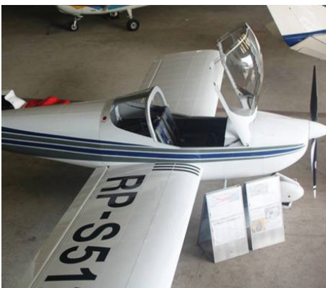
The RP-S512, a locally-assembled light sport airplane with removable wings
