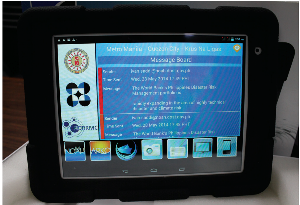
The MOSES tablet - an 8-inch Internet-based, two-way communication tool between warning agencies and disaster responders developed by the Department of Science and Technology's Project NOAH. Aside from its selection as pilot area for Project NOAH, Marikina also became the first recipient of this new tool with 20 tablets handed over to the local government unit. ( S&T Media Service )
