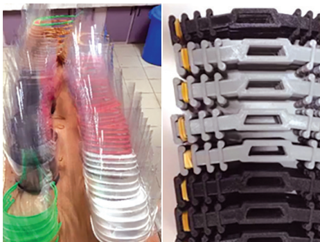
Face shields and ear relief bands in 3D print designs. (Photos courtesy of DOST-ITDI)
