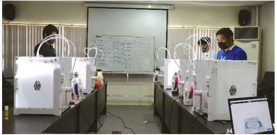
3D printing of RAPPID-ADMATEC face shield frames for use of health workers
