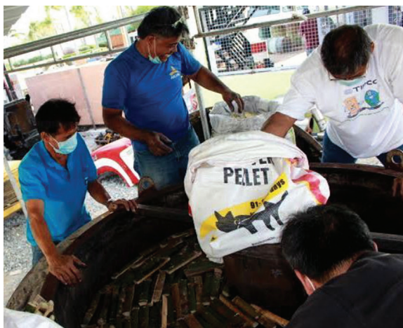
The improved bamboo charcoaling kiln can produce more bamboo charcoal and pyroligneous liquor than the old model.
