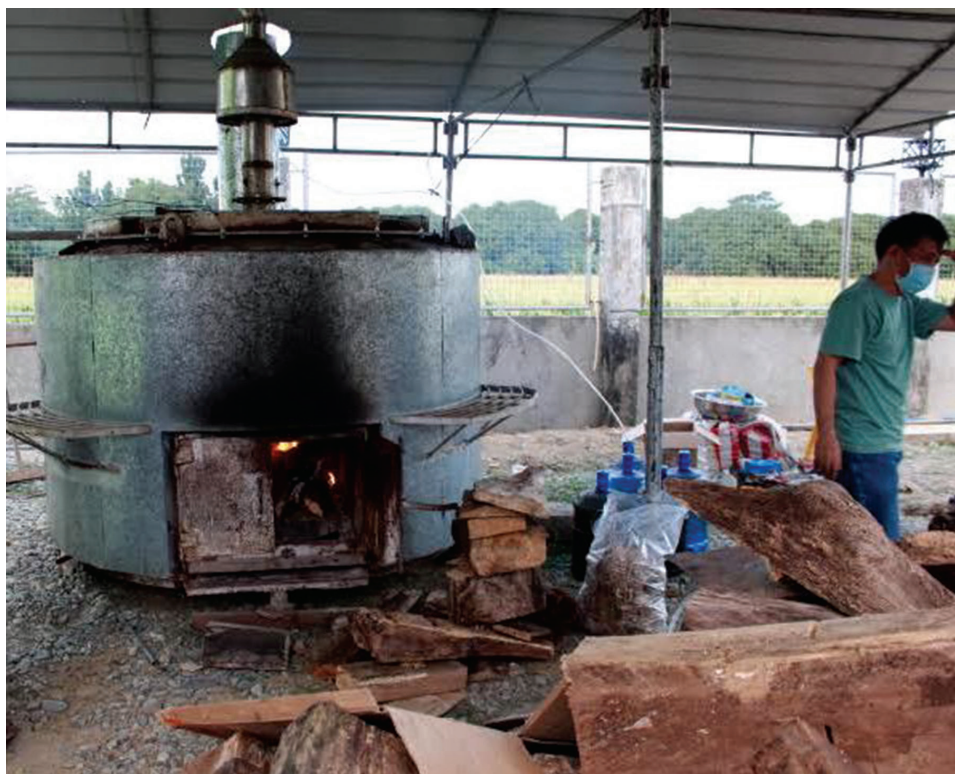
The improved bamboo charcoaling kiln can produce more bamboo charcoal and pyroligneous liquor than the old model.
